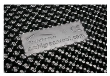
SedumDrain® 25 is the result of extensive research and testing in the quest for the optimal water reservoir and drainage layer for green roofs. The outcome is an unmatched 25 mm high, lightweight water retention and multi-level drainage board, manufactured from recycled high impact polystyrene (HIPS) and is black in colour. The surface is thermoformed on both sides with unrivalled centralised perforations on the top.
